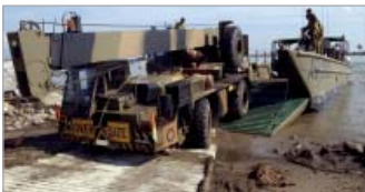
Ground Improvement Mat
