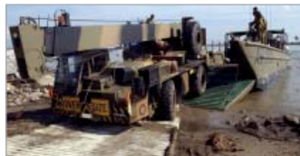
Ground Improvement Mat
